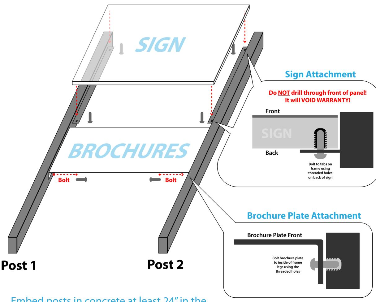
Embed posts in concrete at least 24" in the ground and brace while the concrete sets.
