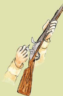
4. Pull the hammer to fully-cocked position.
